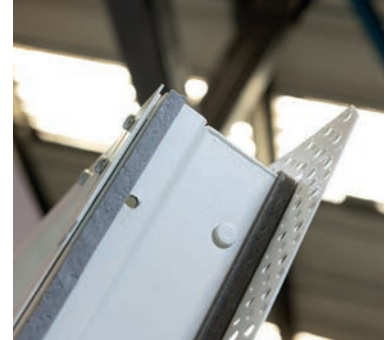
Factory applied intumescent strips eliminate the need for intumescent mastic application.
